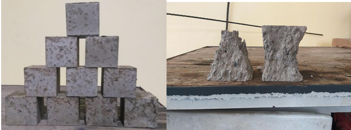
Figure 1. Appearance of concrete cubes and their appearance after compression testing.
