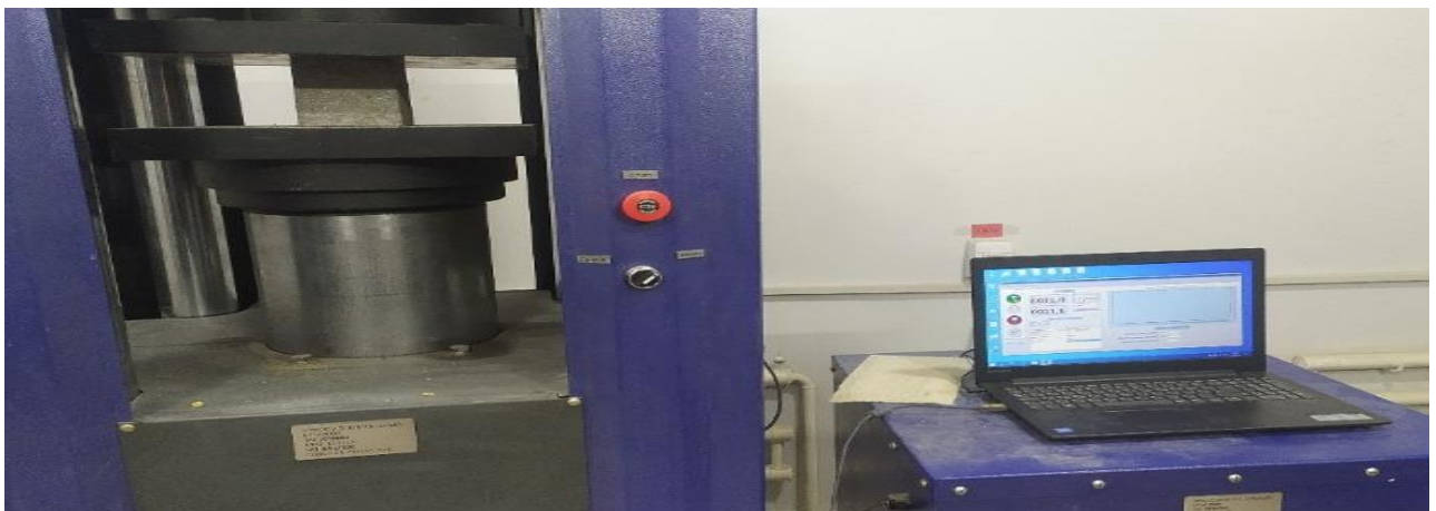
Figure 2. The process of testing concrete cubes for compression.
