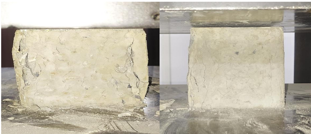
Figure 3. Appearance of cracks in concrete cubes after compression testing.
