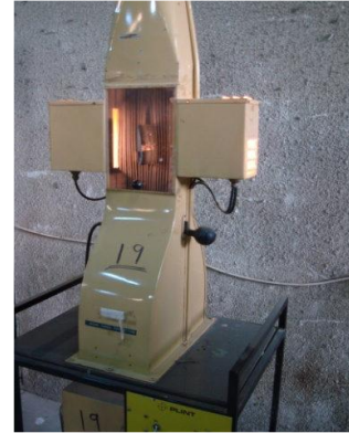
Figure (3) smoke wind tunnel.
