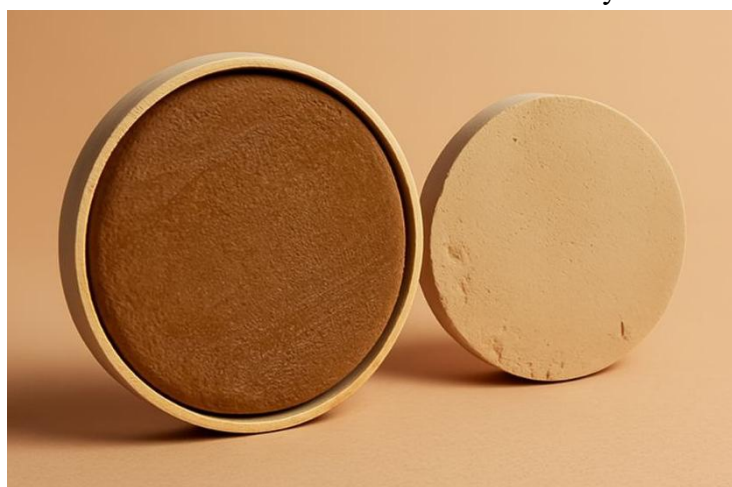
Fig. 7 Views of Karbala clay-sawdust membrane: (a) unsintered membrane and (b) membrane sintered at 1050 °C.
