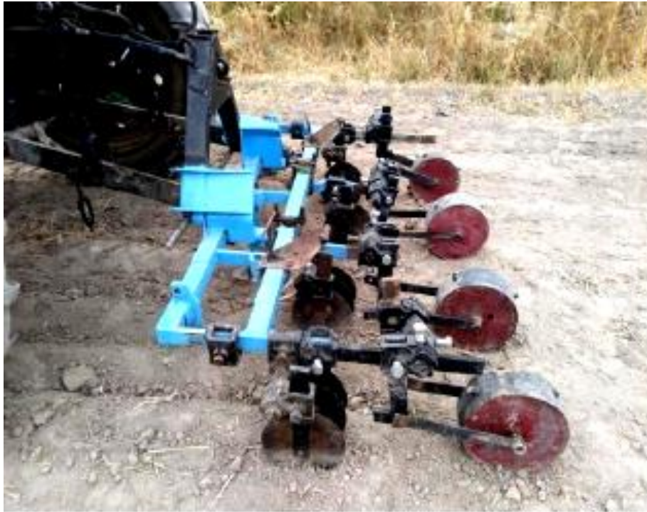
Figure 2 shows an image of a combination unit with a seeder-roller in the proletarian process.
