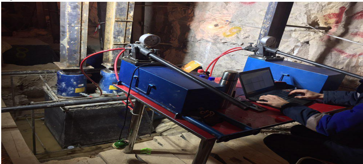
In the photo.1. concrete dies BSh-7 prepared for shear tests are shown.
